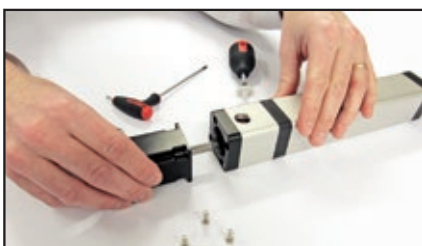
Insert motor shaft into coupling
